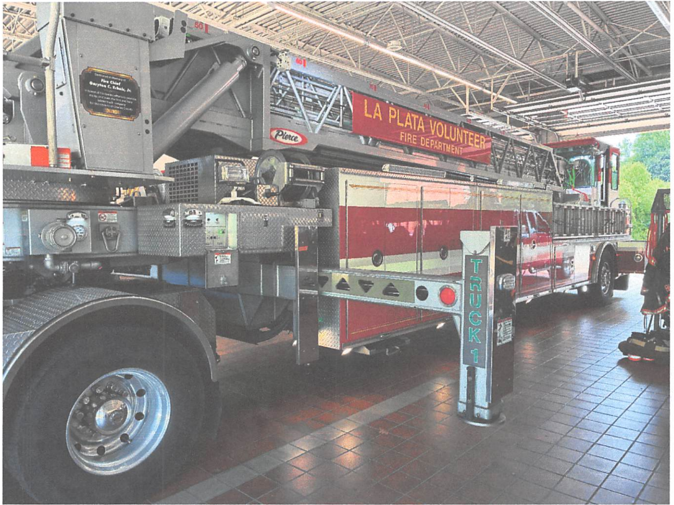
Fire Truck-Trailer Stabilizers Protect Approximately 5 feet from the Vehicle
