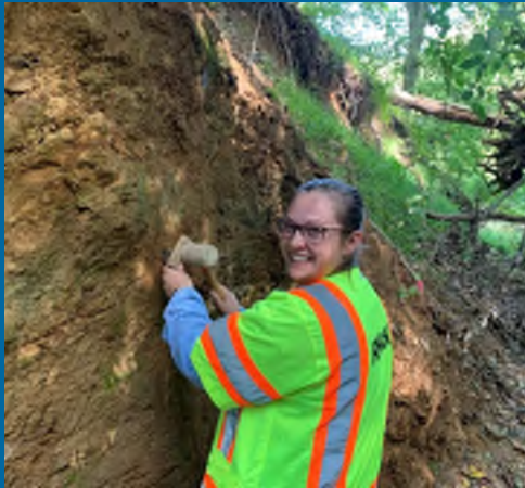
Brittany Ayers collecting soil samples for protocol 5 utilized for outfall gully and stabilization.
