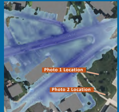
Turner Station Flood Resiliency Study - Model verification using rain full and tidal data in coordination with photo documentation from the community.
