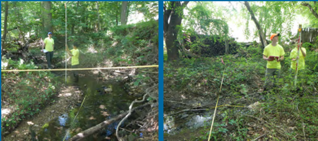
RK&K team performing longitudinal profile and cross-sectional survey at Woodland Run Stream Restoration Project.
