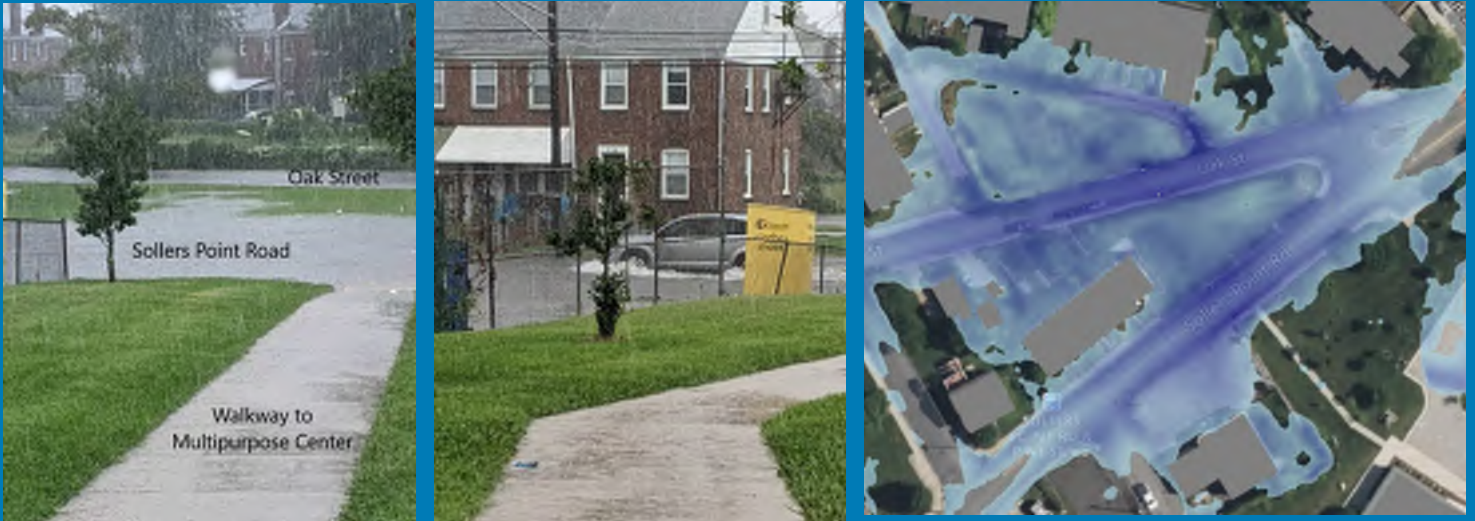
Turner Station Flood Resiliency Study – model verification using rainfall and tidal data from nearby gauges in coordination with photo documentation from the community.
