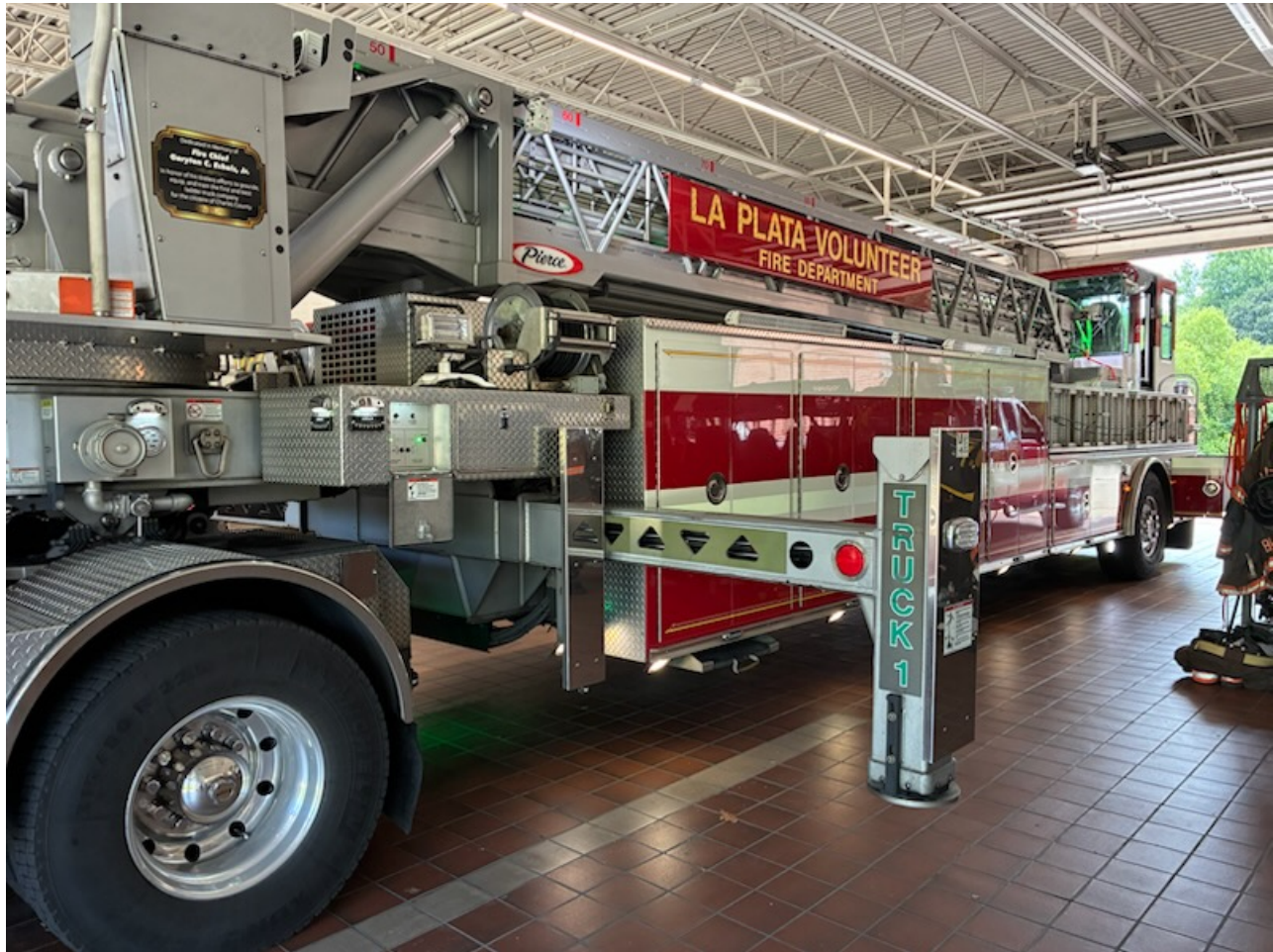
La Plata Fire Truck-Trailer measuring 9-foot wide by 60-foot long (not including side view mirrors). The five-foot wide stabilizers protrude five feet on each side of the vehicle for use of the attached fire ladder.
